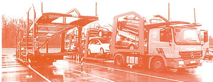
With a special trailer and a slightly modified articulated lorry this concept is also applicable to the transport of vehicles. The trailer is loaded by specialized personnel at the plant or in a compound, the
